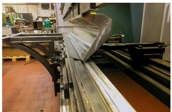
Sheet Metal Bending Machine
